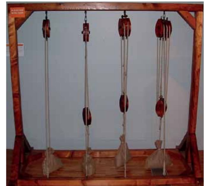
Examples of simple block and tackle pulley systems from the Smithsonian display in Washington DC.
