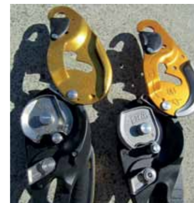
ABOVE: The old (left) and the new (right) ID-S showing the change in cam design and the reinforced stainless steel edge or ridge. BELOW: The stainless 'ridge' and top V-channel on the ID EVAC on the left against an old Petzl RIG on the right with no V-Channel on the top rope-contact surface and the edge of the top plate rolled into a 'wave'.
