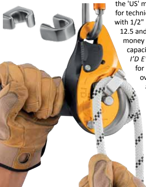
BELOW: The ID EVAC in lowering mode. INSET: the two additional friction hooks. The open hook is standard on the EVAC and both are options on the S&L models.
