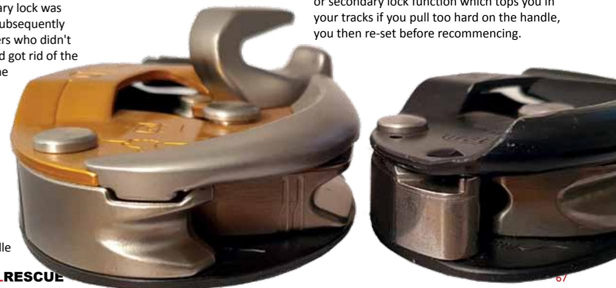
ABOVE: The old (left) and the new (right) ID-S showing the change in cam design and the reinforced stainless steel edge or ridge. BELOW: The stainless 'ridge' and top V-channel on the ID EVAC on the left against an old Petzl RIG on the right with no V-Channel on the top rope-contact surface and the edge of the top plate rolled into a 'wave'.
