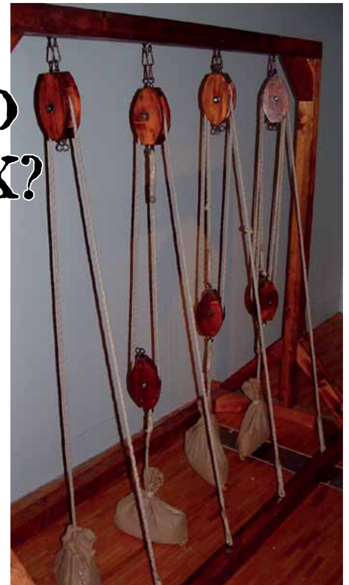
Examples of simple block and tackle pulley systems from the Smithsonian display in Washington DC.
