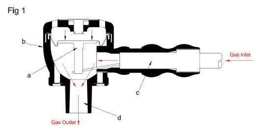
The demand valve has been specifically designed to be used with low-cost single use generic mouth piece and filter systems that are widely available using standard connections that conform to BS EN ISO 5356-1.
